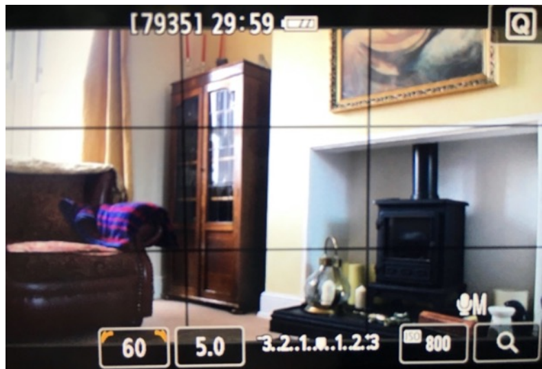
Fig. 11. Adjusting the exposure on a DSLR camera: (from left) shutter speed, aperture, exposure compensation, ISO
