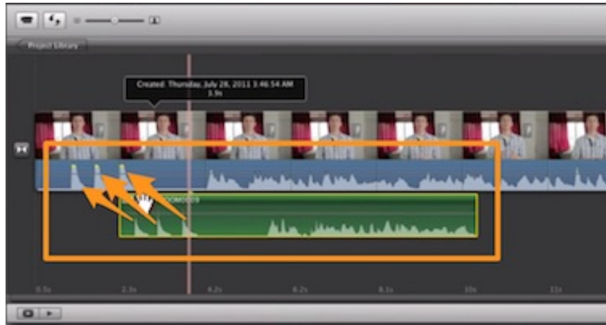
Fig. 16. Syncing externally recorded audio (green) with video (blue) by lining up claps, or the closing of the slate.
