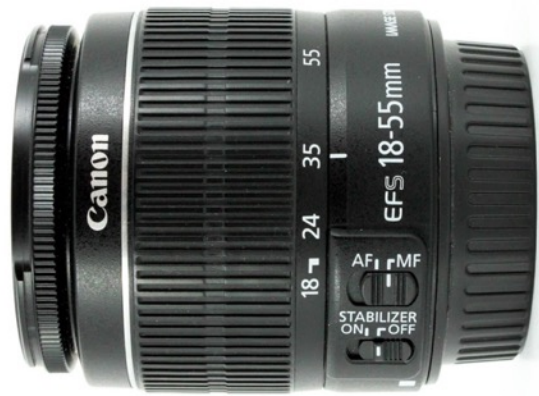
Fig. 13. Canon 18-55 zoom lens showing auto/manual focus buttons and focus ring (far left).
